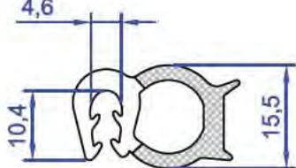
Clamping Thickness 2.5mm
