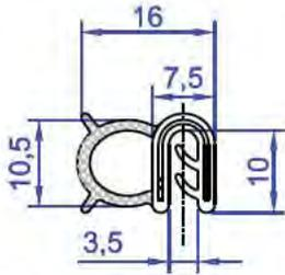
Clamping Thickness 2mm
