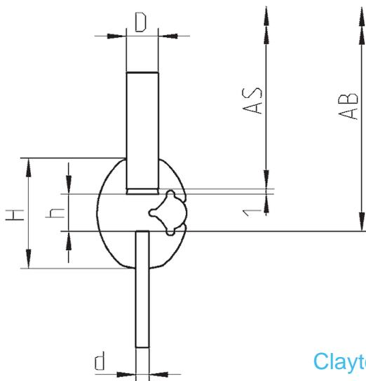
Claytonrite glazing profiles with locking insert
